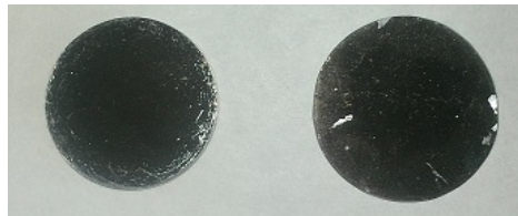
Figure 4.3: Photograph of two different matte black painted samples, (left) before heating, and (right) after heating.
